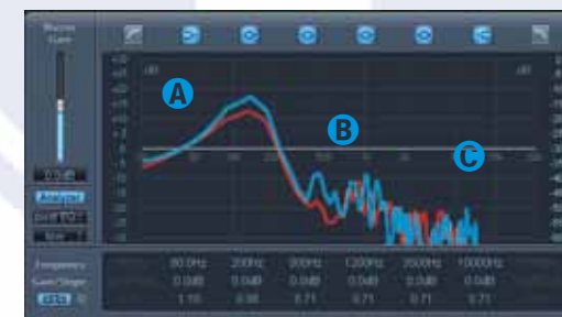
18X22” BASS DRUM WITH & WITHOUT BASS PLATE
